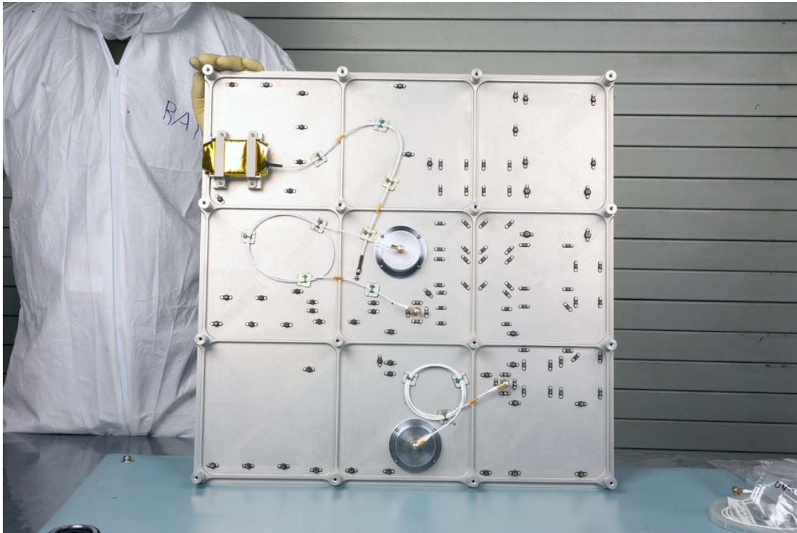
Figure 6 Post-flight image of underside of baseplate showing oxidation on the silver-coated nut plates (NASA Image)
