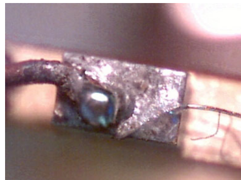
Figure 12: Ceramic Pad on Package Top
