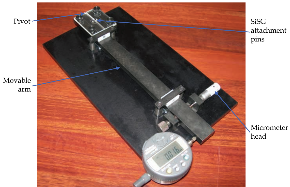
Figure 3: Micro-Displacement Rig designed for manual characterisation of Silicon Strain Gauges.
