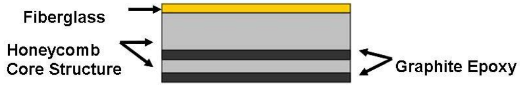
Figure 11 Conformal Load-bearing Array Structure (CLAS)
