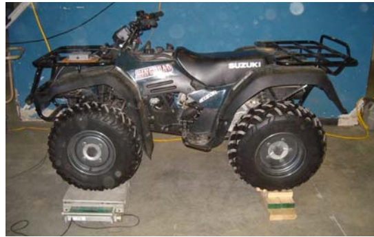
Figure 3. Side view of the ATV sitting level with scales under the front tires.
