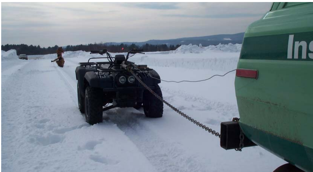
Figure 14. ATV rolling resistance test on snow.
