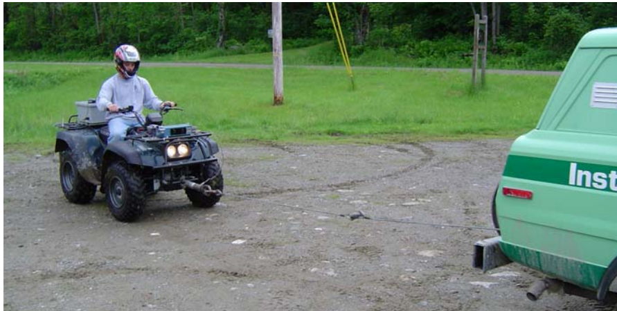
Figure 13. Conducting a rolling resistance test on the ATV.
