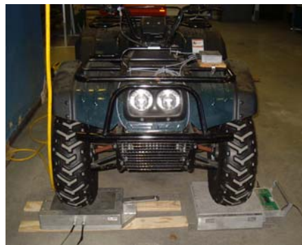
Figure 4. A front view of the ATV with scales under the front tires.
