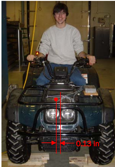
Figure 5. ATV's Y center of gravity location.
