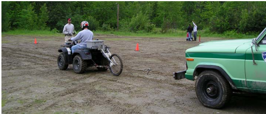
Figure 12. The ATV pulls the CIV during a traction test at EAFR.
