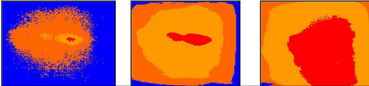
Figure 9: Graphics of thermal impedance testing at 600 W of neat foam at 3.5 and 2.0 gpm and a coated sample at 2.0 gpm.
