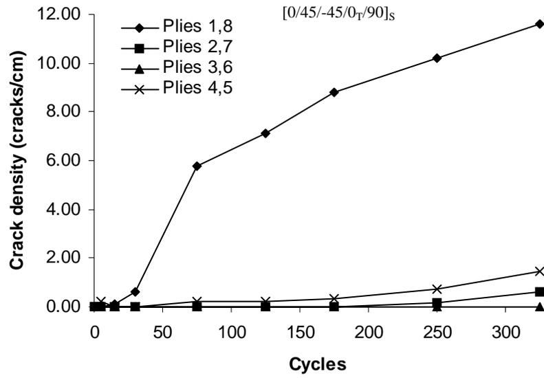
Figure 5: Micro-crack density versus -196 °C to 177 C cycles in IM7 / 5250-4 [0/45/-45/0<sub>T</sub>/90]<sub>S</sub> samples
