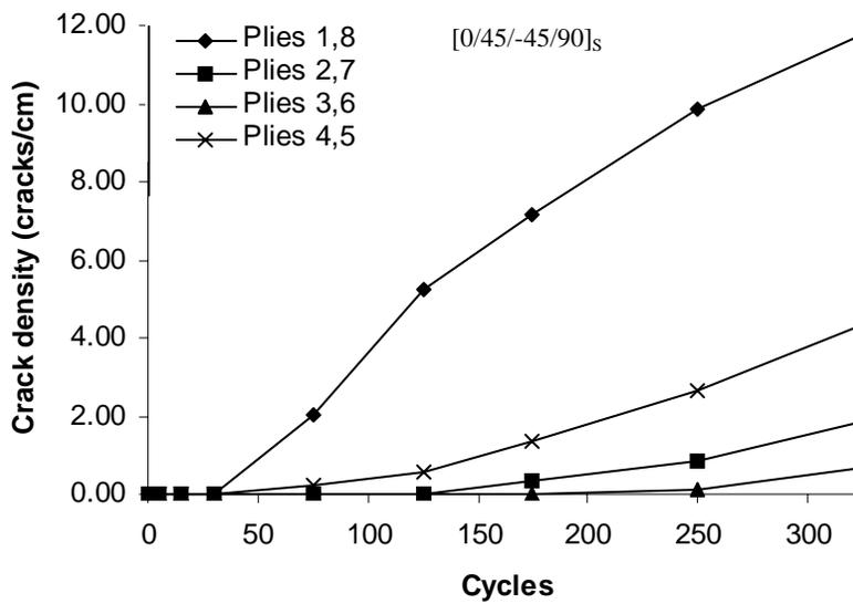
Figure 4: Micro-crack density versus -196 °C to 177 °C cycles in IM7 / 5250-4 [0/45/-45/90]<sub>S</sub> samples
