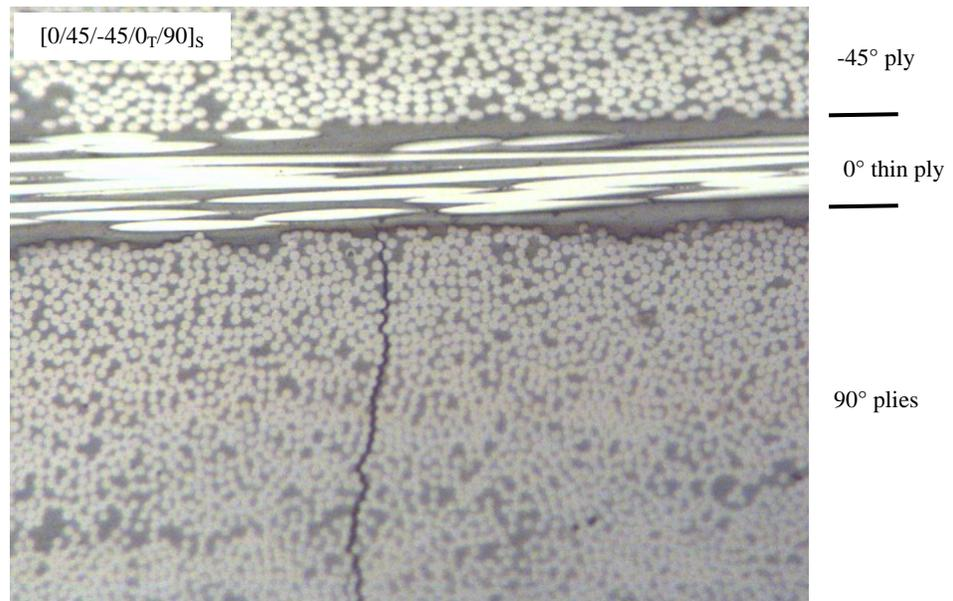
Figure 6: Crack in 90° ply group of [0/45/-45/0<sub>T</sub>/90]<sub>S</sub> sample stopped at the interface with the thin ply
