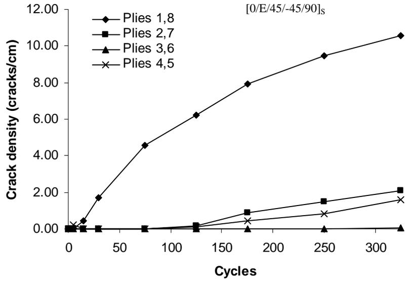
Figure 11: Micro-crack density versus -196 °C to 177 °C cycles in IM7 / 5250-4 [0/E/45/-45/90]<sub>s</sub> samples
