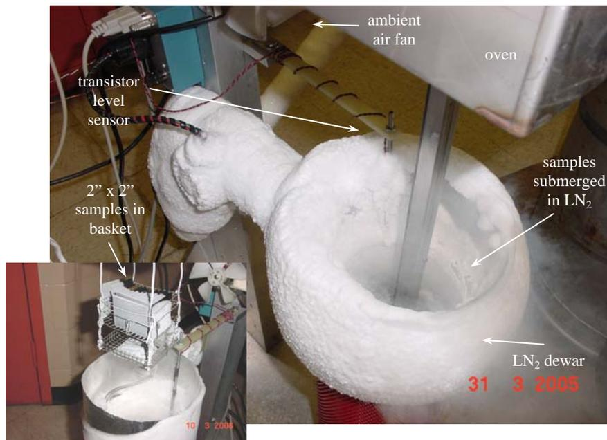
**Figure 2: Cryogenic and elevated temperature thermal cycler**
