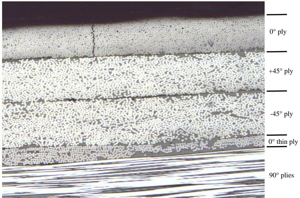
Figure 3: Image showing thin ply in IM7 / 5250-4 [0/45/-45/0<sub>T</sub>/90]<sub>S</sub> lay-up
