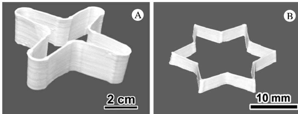
Figure 10: Optical images showing sintered thin walled polygon components produced from  $\text{Al}_2\text{O}_3$ . Part "A" was fabricated with a 580  $\mu\text{m}$  diameter nozzle and "B" was fabricated with a 250  $\mu\text{m}$  diameter nozzle.
