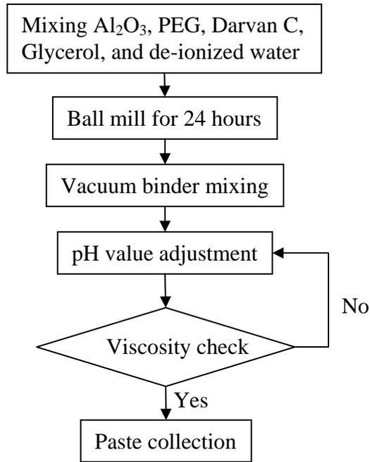
Figure 1: Flowchart for the paste preparation process.
