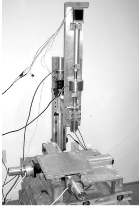
Figure 2: The FEF 3-D extrusion-deposition system.
