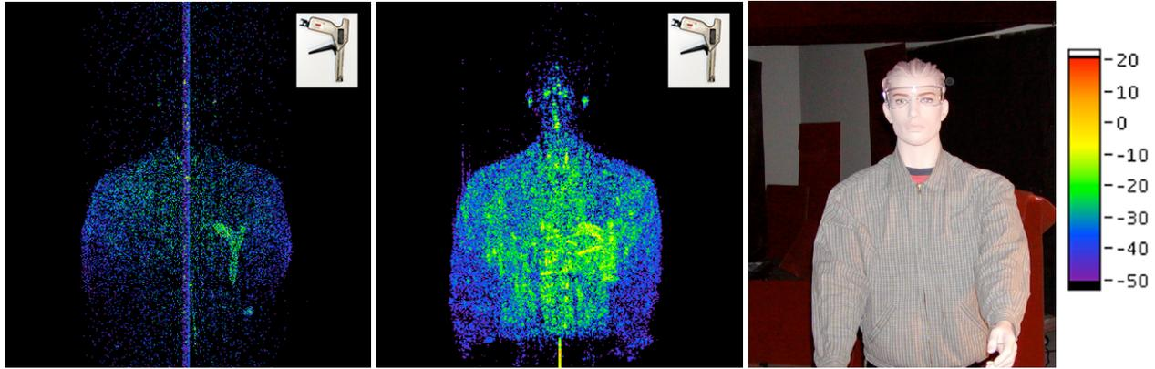
Figure 3.1. Azimuth/elevation collection of a clothed mannequin with a concealed, metal tie-wrap "gun"(inset). Left image taken at 1.56THz. Center image taken at 350GHz (dBV<sup>2</sup> color scale). Photograph of subject as measured on right. Note the penetration through the black plastic wrapping of the trigger handle at 350GHz. The black plastic wrap is heavily attenuating at 1.56THz and minimally attenuating at 350GHz, allowing the handle metal to reflect brightly.
