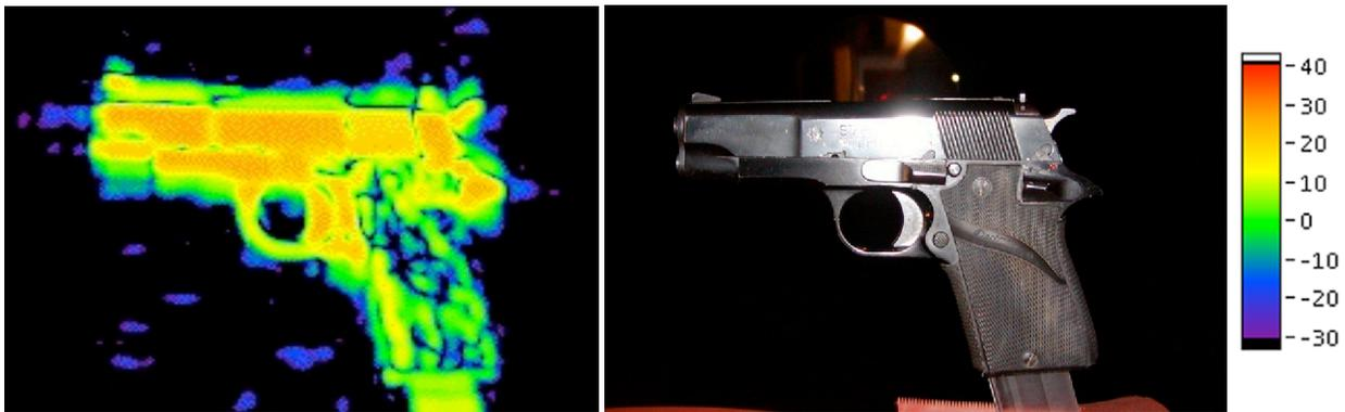
Figure 3.2. A 350GHz Az/EI image (left) of a .45 Caliber handgun and a photograph of the measured gun (right) (dBV<sup>2</sup> color scale).
