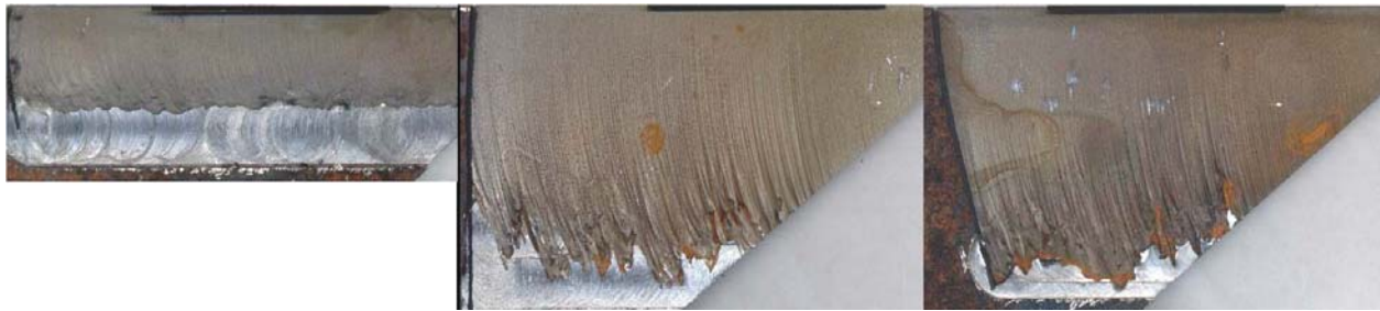
Figure 1. Section showing the cut made by three different abrasive jets at the same AFR, speed and pressure.
