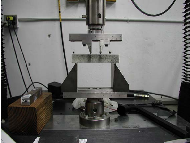
Figure 5: Four point bend fixture with 6"x1"x1" specimen prepared for DIC
