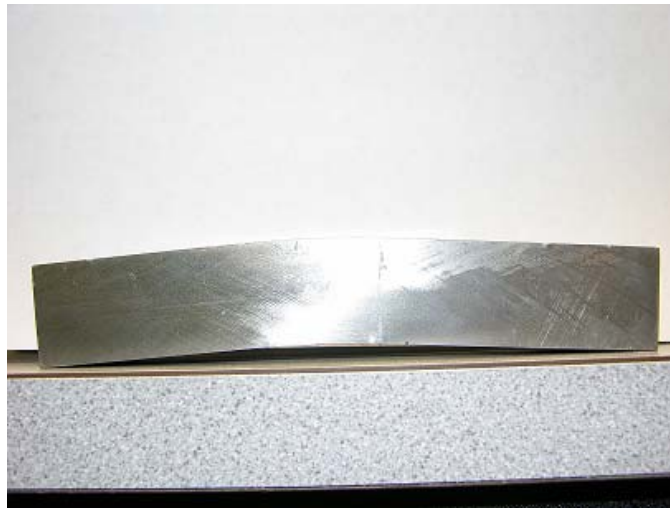
Figure 8: Deformed uniform Ti specimen after loading
