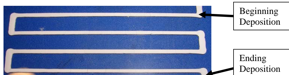
Figure 3: Deposition lines using extrusion force controller.
