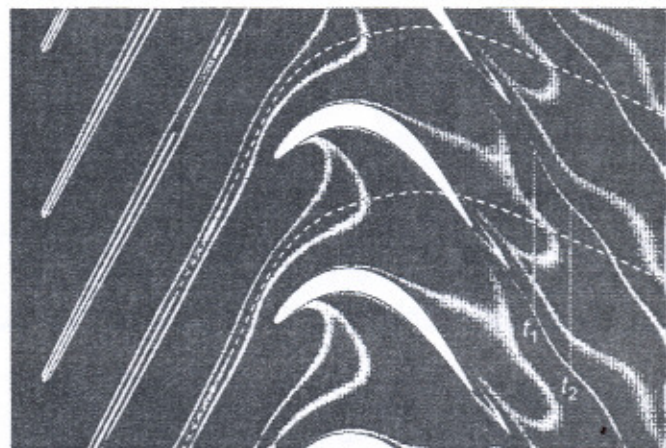
Figure 9. Instantaneous entropy distributions with superimposed time-mean wake paths (in the wake-generation reference frame) for the stage simulation with WVR=0.56 .
