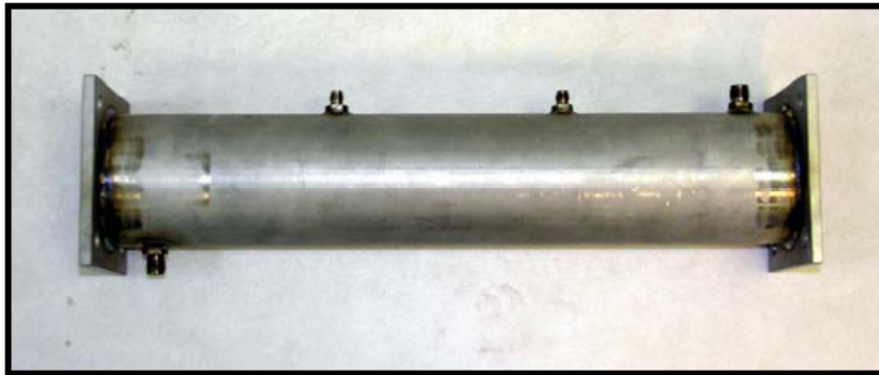
Figure 26. Photograph of 15 inch heat exchanger
