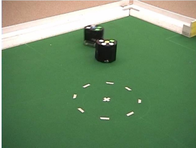
Figure 6.1: Keepout: an adversarial robot task. The top robot is trying to get inside the circle while the bottom robot is trying to stop it.
