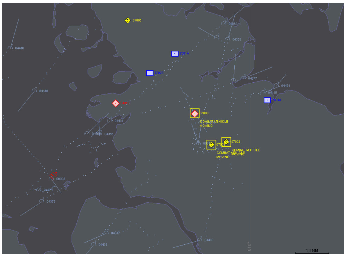
Figure 6 Simulated J3.5 track messages over real targets on live tactical display
