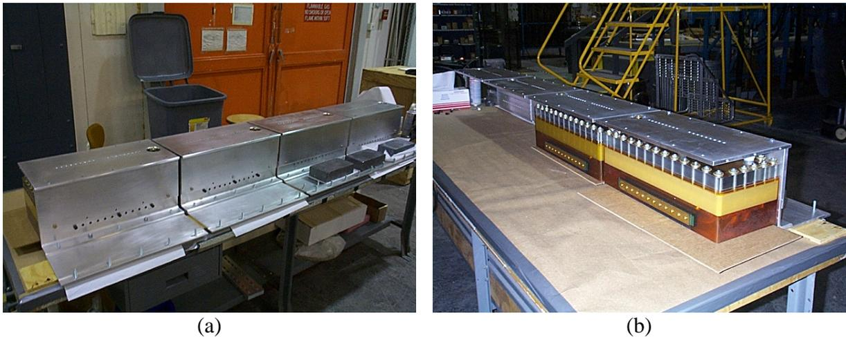
**Figure 51. Photos of (a) the bank side and (b) the Theta coil side of the new Crowbar switch slotted bus work during its test fitting. As is shown in (b), two single rail-gap switches were set out and spaced appropriately to allow the bolt-hole spacing and the sizes of parts to be checked.**
