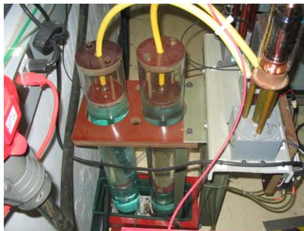
**Figure 22. Photo of one of the charge and dump resistor stands, with the Jennings charge and dump switches mounted to it (upper right), on the FRX-L experiment. Bank voltage monitors are also mounted on these stands.**
