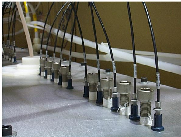
**Figure 11. Photo showing the fiber optic cables in the aluminum bus plate over one of the Crowbar rail-gap switches. Simplex fiber optic feed-throughs in the plate hold the fibers in place – ten per switch. Socket head bolts are used to plug the empty holes.**
