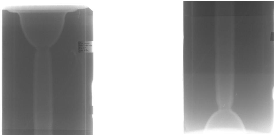
**Figure 34. Radiographic image of the liner taken 20.96  $\mu$ s after current delivery began.**
