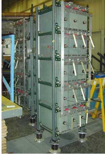
**Figure 15. Photo of two of the “Slow Bank” modules that have been set in place between Shiva B and C Arms for use in the FTX experiment. The module in the foreground is intended for use in the Bias bank circuit, while the one in the background (and others still in storage) will be used for the other slow banks (Cusp, Guide, or Mirror).**
