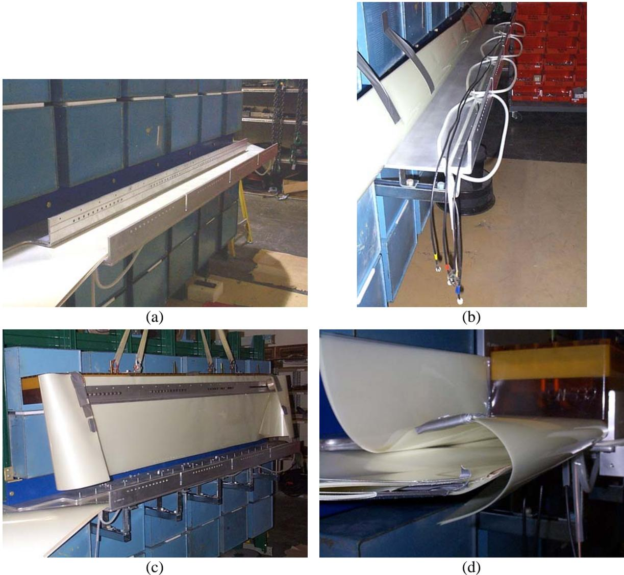
**Figure 9.** (a) The Mylar packs from the Main bank stretched out uniformly on the ground plate below the Crowbar switch; (b) Crowbar and Main-bank Rogowski coils shown in place around the load-side Crowbar supports and the bottom-bus plate, respectively; (c) The Crowbar rail gaps suspended and rotated 180° so that the small Mylar pack can be affixed to its side; (d) the Crowbar switch Mylar is wrapped around the bank Mylar packs as the Crowbar switch is lowered into place.
