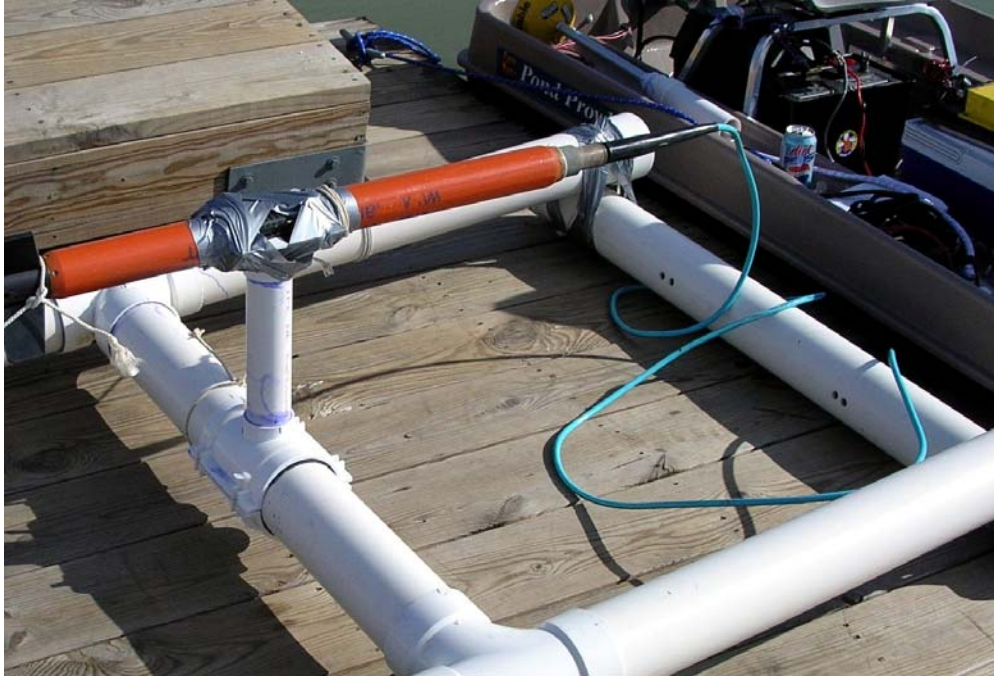
Figure 3. MM Explorer mini proton-based magnetometer.
