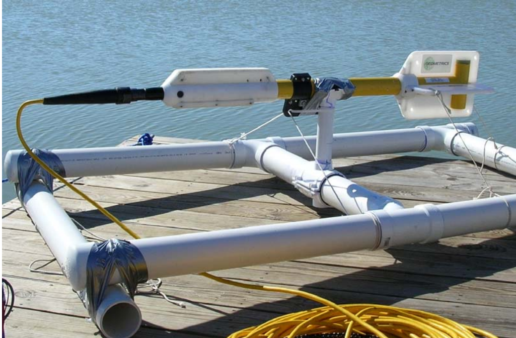
Figure 2. G882 cesium-based marine magnetometer.
