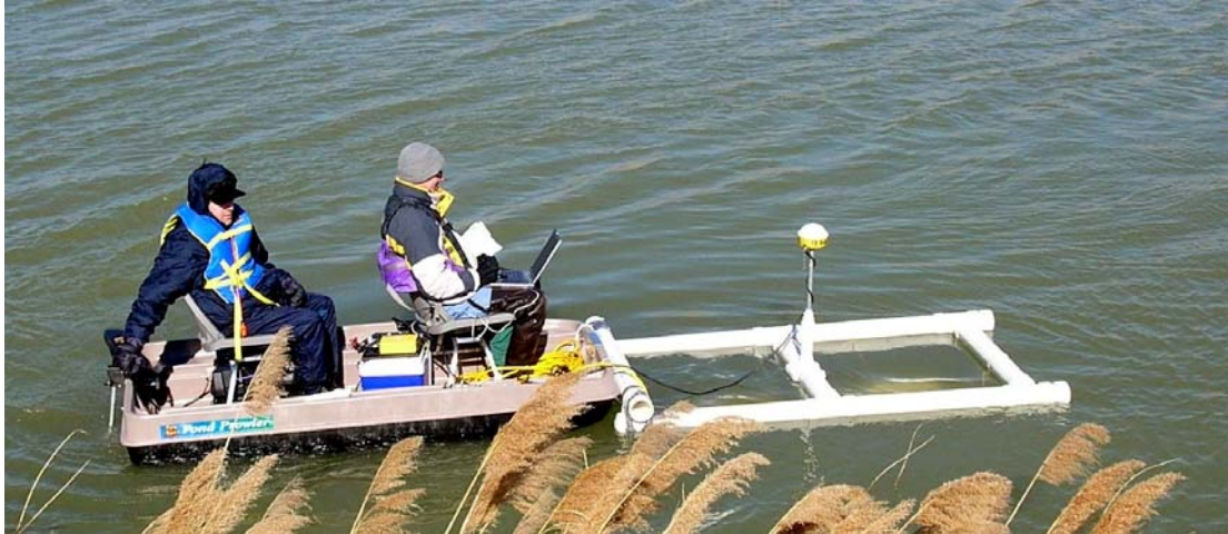
Figure 4. IT Jewell's shallow water UXO detection platform.
