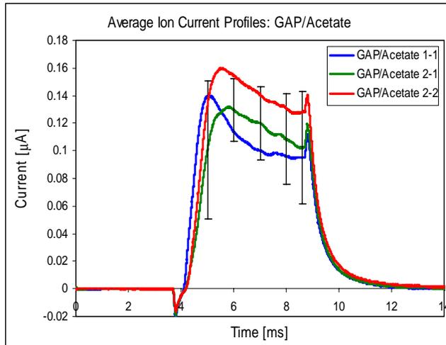
**Figure 11. GAP/Acetate average ion currents.** The traces are for 24.5mJ deposited over 5ms. GAP/Acetate 1-1 represents one sample taken from fuel strip #1, whereas 2-1 and 2-2 indicate samples 1 and two taken from a separate fuel strip.
