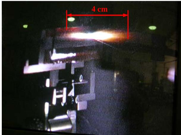
**Figure 5. Photo of First 3 milliseconds of  $\mu\text{LPT}$  discharge.** Here the plume is visually estimated to be about 4 centimeters long.
