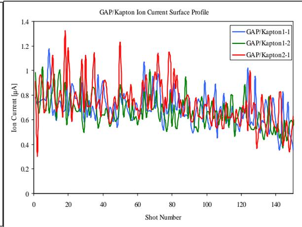
**Figure 15. GAP/Kapton average ion currents.** The traces are for 24.5mJ deposited over 5ms. Traces were taken at 150 successive fuel locations. GAP/Kapton 1-1 represents one sample taken from fuel strip #1, whereas 2-1 and 2-2 indicate samples 1 and two taken from a separate fuel strip.
