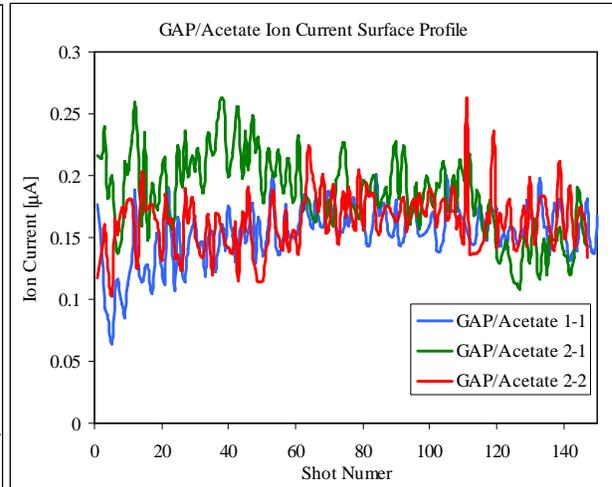
**Figure 12. GAP/Acetate average ion currents.** The traces are for 24.5mJ deposited over 5ms. Traces were taken at 150 successive fuel locations. GAP/Acetate 1-1 represents one sample taken from fuel strip #1, whereas 2-1 and 2-2 indicate samples 1 and two taken from a separate fuel strip.
