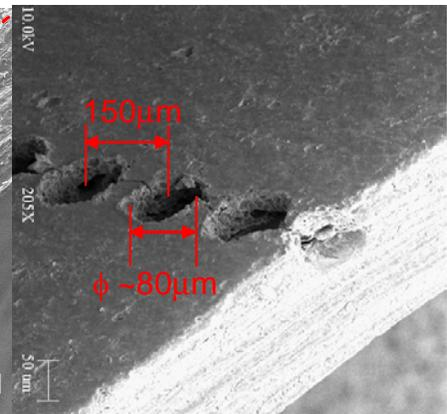
**Figure 16b. PVC/Acetate SEM photo.** The distance between the ablation events and across each crater is observed.
