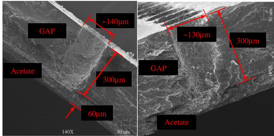
**Figure 10a. GAP/Acetate SEM photo. Figure 10b. GAP/Acetate SEM photo.** This The target/substrate thickness and depth is a different ablation crater than Figure 10a but similar results are observed.
