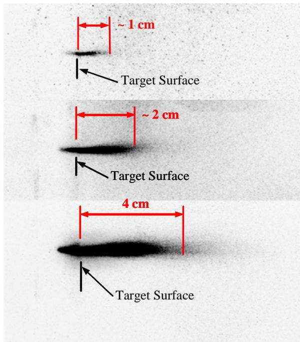
**Figure 6. Plume Expansion from Target Surface.** All plumes are due to 24.5 mJ of deposited laser energy over 5 ms. Therefore, the topmost plume shows the smallest amount of ablated material being ejected. The average length of plume expansion during the first millisecond was observed to be 4 cm.
