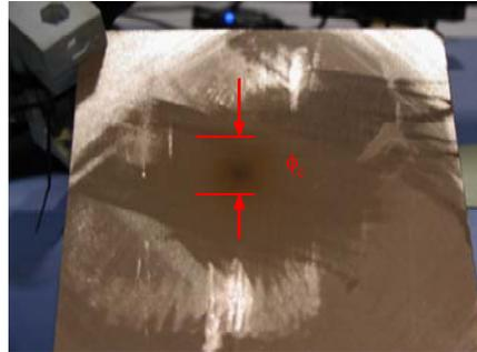
**Figure 7a.  $\mu$ LPT T-mode with copper probe.** The copper probe was negatively biased with a 9V battery and ion currents were measured with secondary electron emission neglected.
