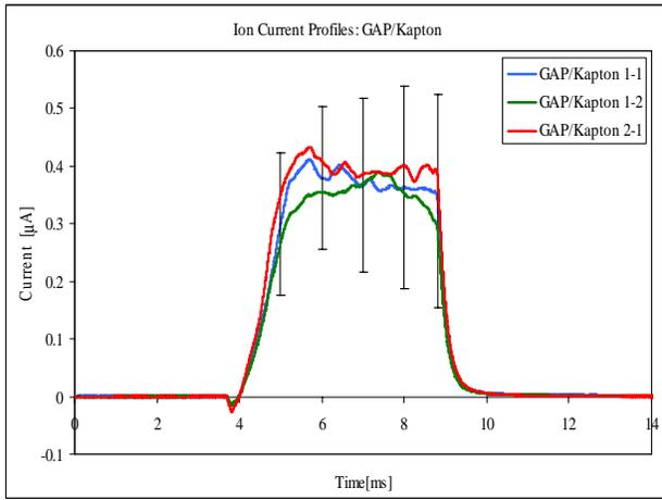
**Figure 14. GAP/Kapton average ion currents.** The traces are for 24.5mJ deposited over 5ms. GAP/Kapton 1-1 represents one sample taken from fuel strip #1, whereas 2-1 and 2-2 indicate samples 1 and two taken from a separate fuel strip.
