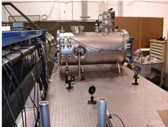
**Figure 2. Vacuum system setup used in testing.** *The chamber is seated on a 120x300x30 cm optics table with pneumatic legs.*
