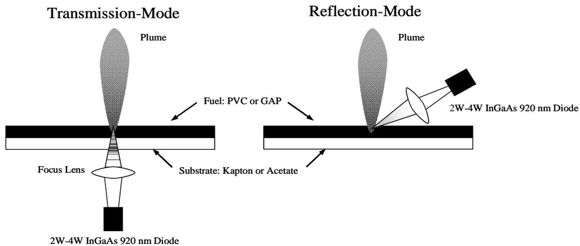
**Figure 1. Transmissive Mode (T-mode) Ablation vs. Reflective Mode (R-mode) Ablation.** *T-mode ablation protects the system optics but suffers from reduction in  $I_{sp}$  and exhaust momentum compared with R-mode. The R-mode, although enabling a greater  $I_{sp}$ , is lifetime restricted due to coating of optics by exhaust material.*
