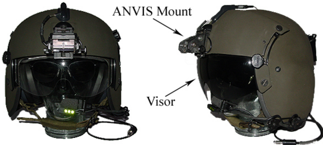
Figure 1. Front view of the HGU-56P helmet showing the ANVIS mount and the tinted visor.
