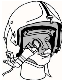
Figure 2. Artist rendering of IHADSS shown with a tinted visor on the outside.
