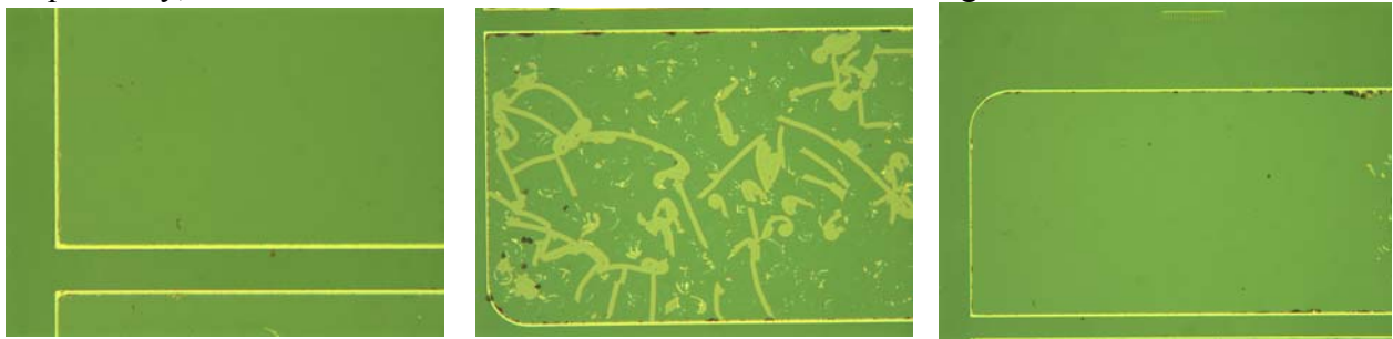
Figure 3-40. SiO 2 under Ti/Pt/Au without and with wire bond after 200 hour aging. Left - SiO 2 under Ti/Pt/Au without wire bonds after 2000 hour of aging. Middle - SiO 2 under Ti/Pt/Au with Au wire bond after 2000 hour of aging. Right - SiO 2 under Ti/TiW/Au with Au wire bond after 2000 hour of aging.
