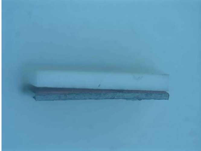
Figure 3-24. Cu foil delamination after 250 thermal cycles.
