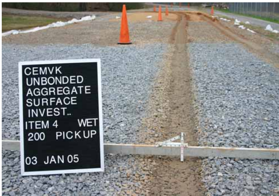
Photo C38. Item 4 (IGN), wet lane, maintenance test section, 200 passes with pickup truck
