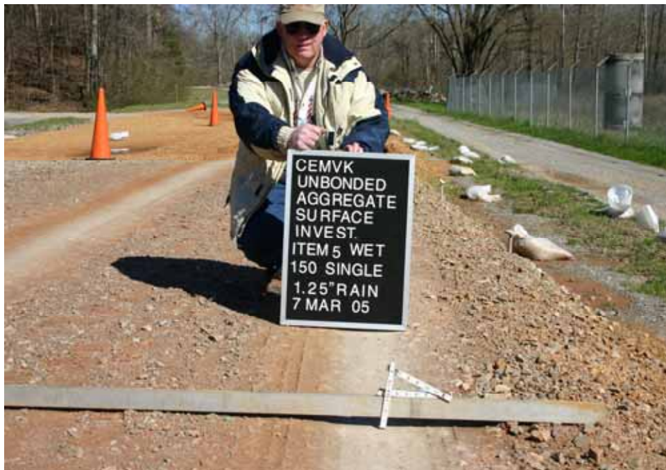
Photo C60. Item 5 (SSB), wet lane, maintenance test section, 150 passes with pickup truck
