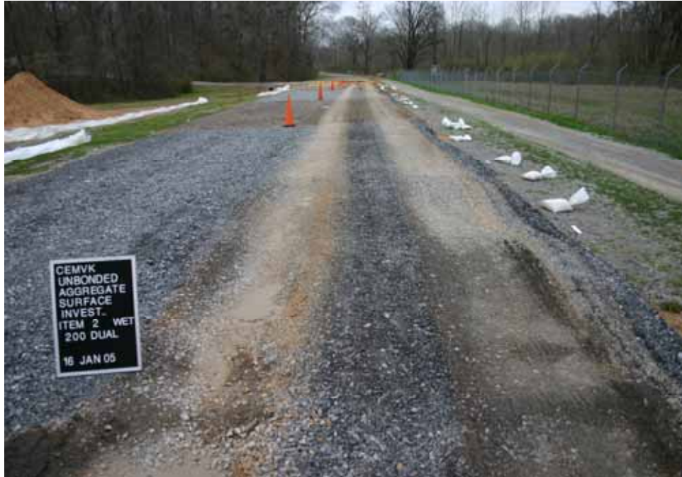
Photo C43. Item 2 (LST), wet lane, maintenance test section, 200 passes with dump truck
