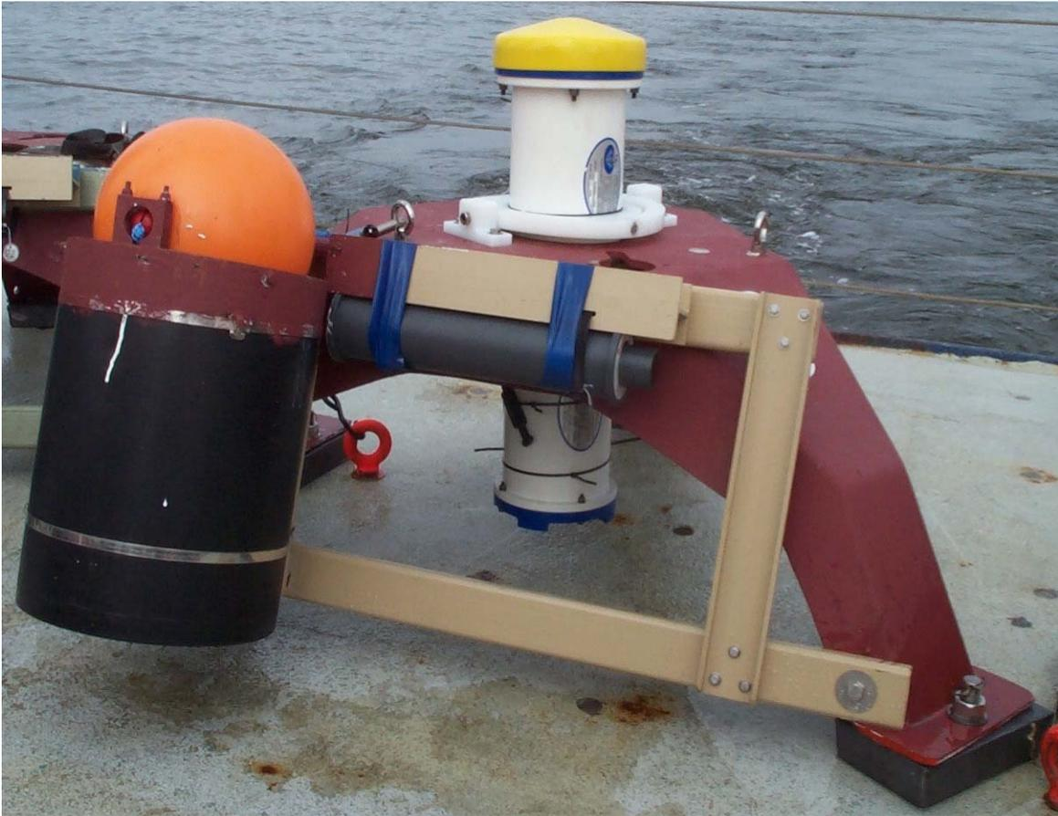
Figure 2. Teledyne Workhorse Sentinel ADCP (upper photo) mounted on Sea-Spider prior to deployment (lower photo). Mounted below the instrument is an extra battery pack. Attached to the front side of the Sea-Spider is the acoustic release assembly with a recovery buoy. (Upper photo from <http://www.rdinstruments.com/sen.html>), Retrieved October 2006.
