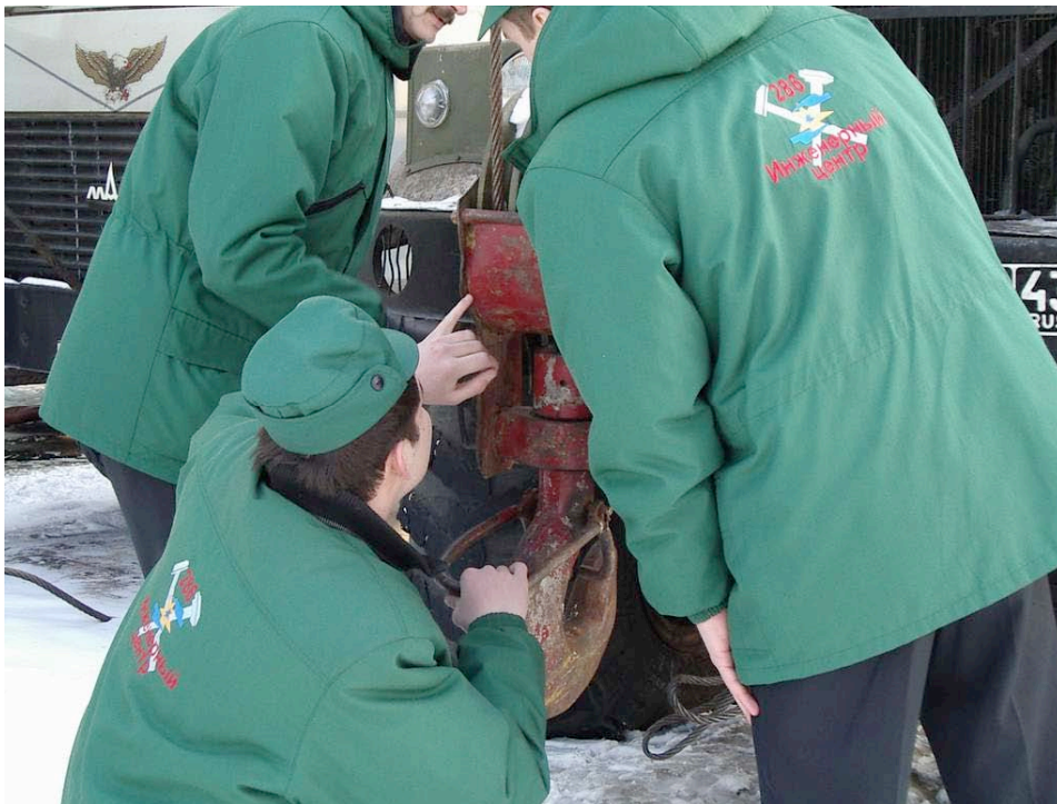
Figure 5.12b: Crane Examination Techniques – Examining the Lifting Pivot.
