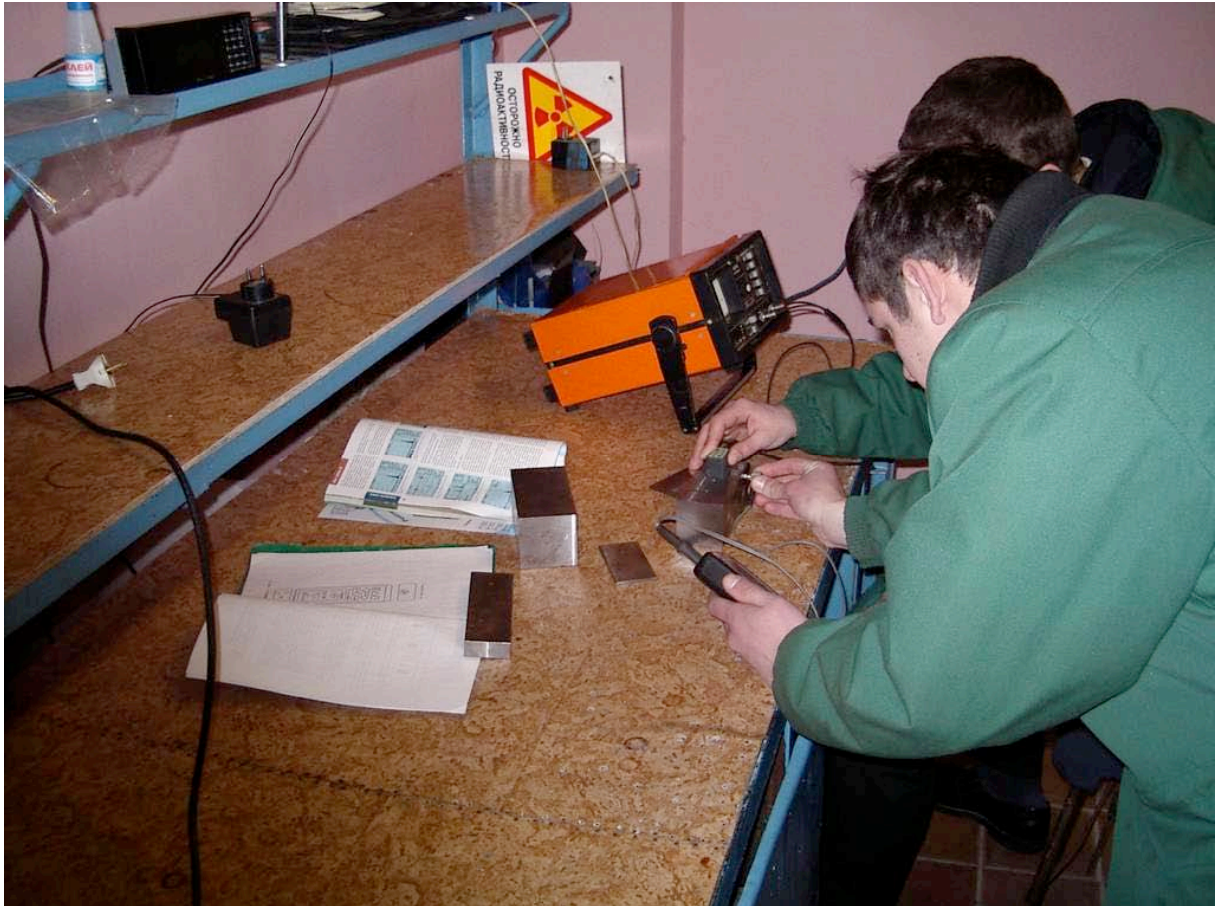
Figure 5.4: Laboratory Procedures for Ultrasonic Identification. In this illustration, the MOD students prepare a laboratory diagnostic report for the test sample using the Russian (Dubeliv) Ultrasonic Defectoscope (Sonatest, Stresstel equivalent). The student is moving a transducer across the test surface as a method to identify internal stresses, cracks, moment deformations, and imperfections. The system requires each student to understand the instrumentation and the proper evaluation techniques for technical reporting and fatigue life estimation.
