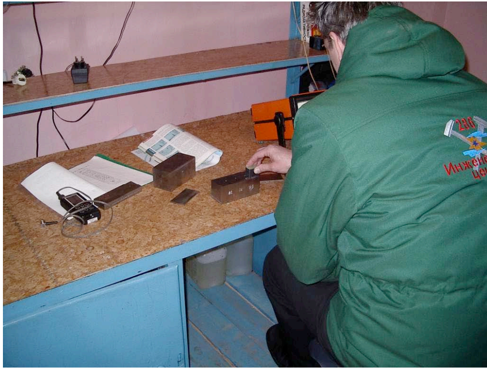
Figure 5.5a: Ultrasonic Flaw Detection. Surface Methods Using Coupled Transducers.
