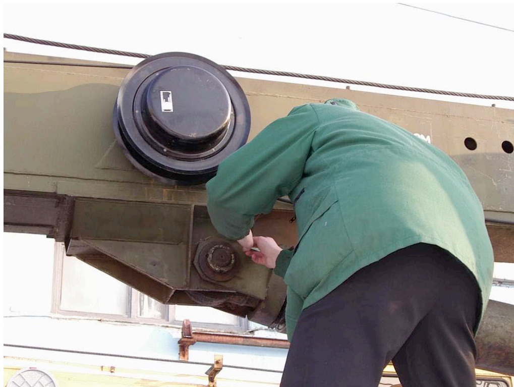
Figure 5.14b: Crane Examination Techniques – Hydraulic Friction Points.
