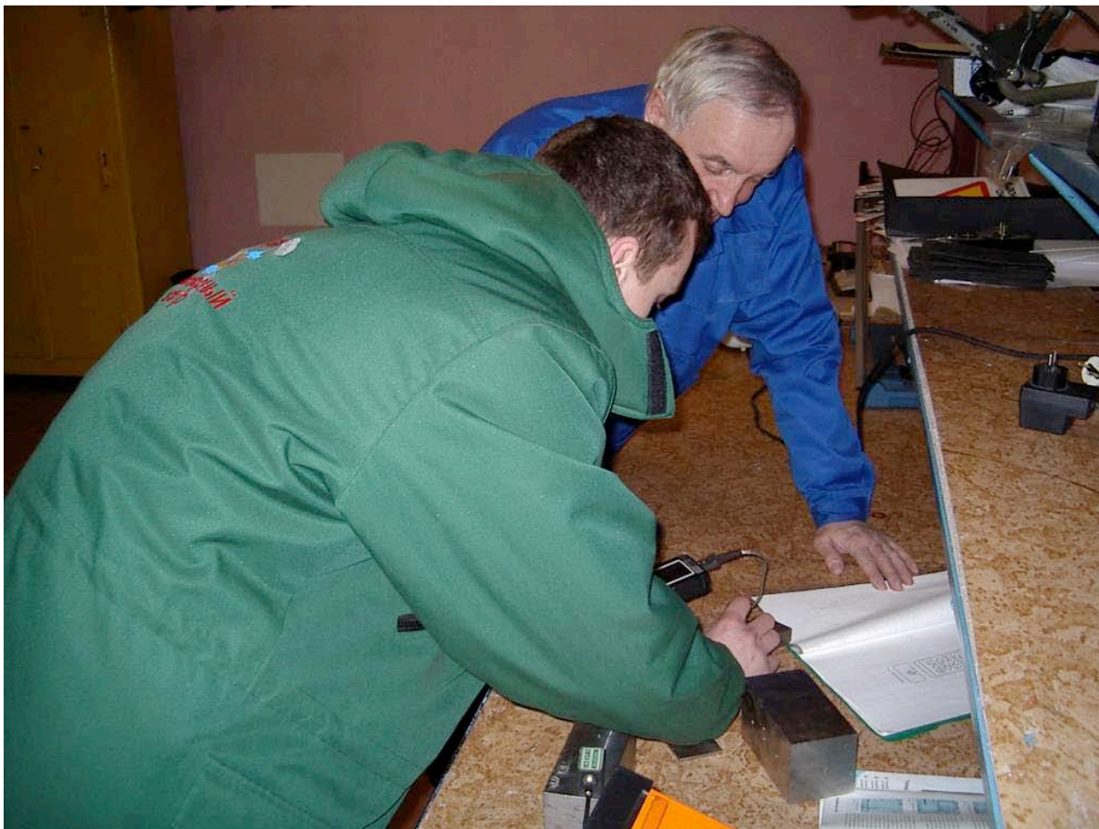
Figure 5.1: Laboratory Certification and Instrumentation Using the StressTel T-Mike EL System. The student receives one-to-one instruction with technical documentation from the manufacturer. The instruction is designed to assist the student in data analysis and data migration methods for the LIMS.
