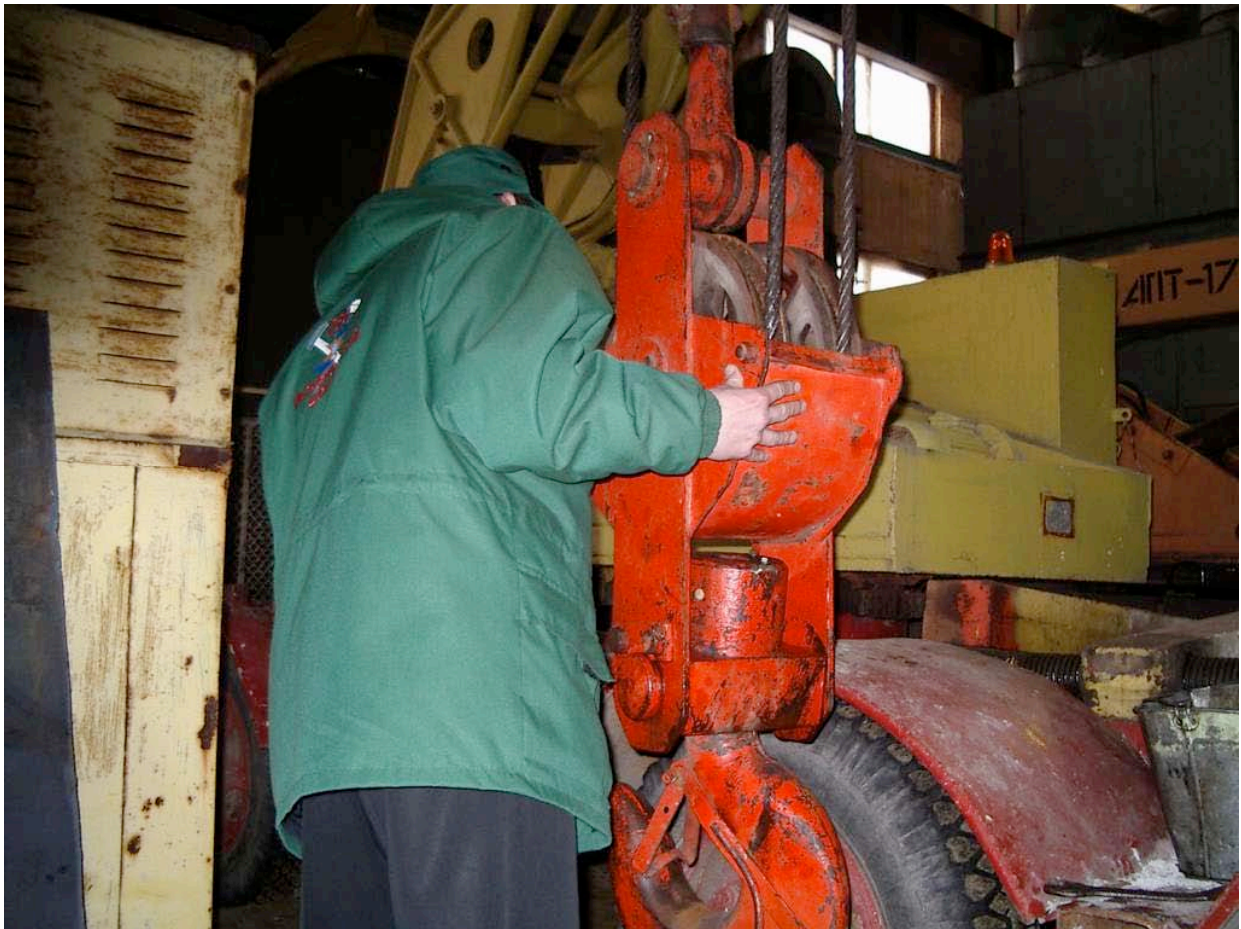
Figure 5.8: Crane Examination Techniques – Cable Lifting Systems. In this illustration the student is working through a prescribed series of surface tests that are required to characterize the functional operating capacity of the crane. These tests are used to develop a working model of how the hoist should be used given the approximate working capacity of the system and the remaining service life of duty cycle for the crane. The student is also shown methods for lubricating the cable system to minimize surface wear and cable friction.
