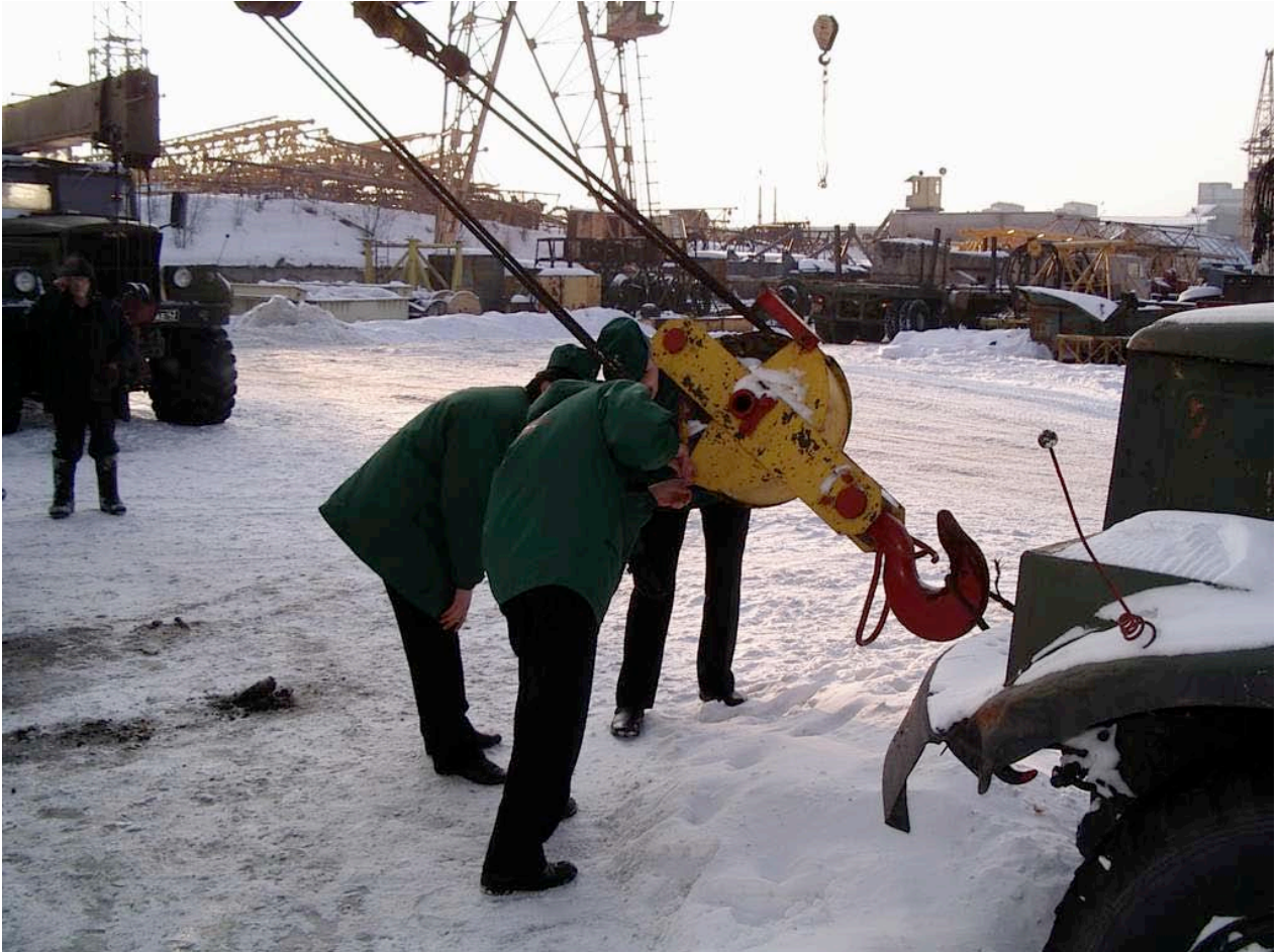
Figure 5.11: Crane Examination Techniques – Load Testing Sequence. In this illustration, the MOD students are preparing the crane for a sequential load test that begins with a static load and ends with a pulsed load of a known weight. The static test is usually designed for 1.8 to 2.2 times above the rated service capacity of the crane. When this test is performed, the cable and hoisting mechanism is gauged to determine the stress induced during the lifting sequence. The pulsed test includes a series of lifts and drops that simulate a jerking process. The pulse generates sharp tensions on the crane cable that may be analyzed for elongation and probable deformation or loss of cross-section.
