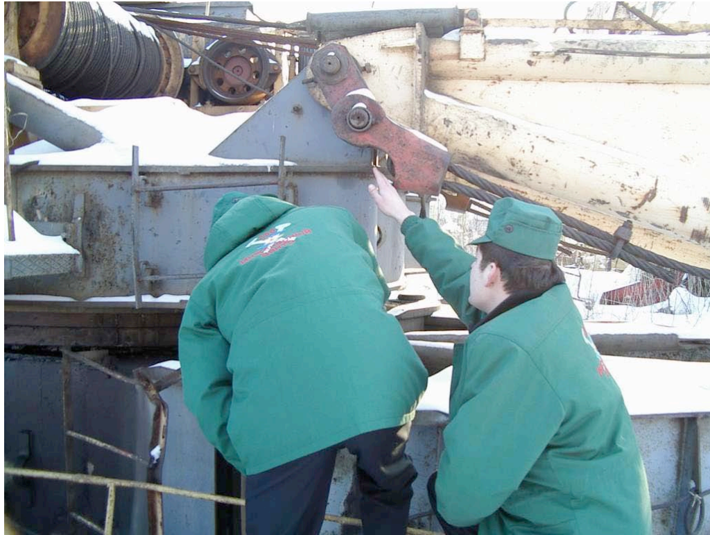
Figure 5.10a: Crane Examination Techniques – Pivot Assemblies and Pinion Systems.
