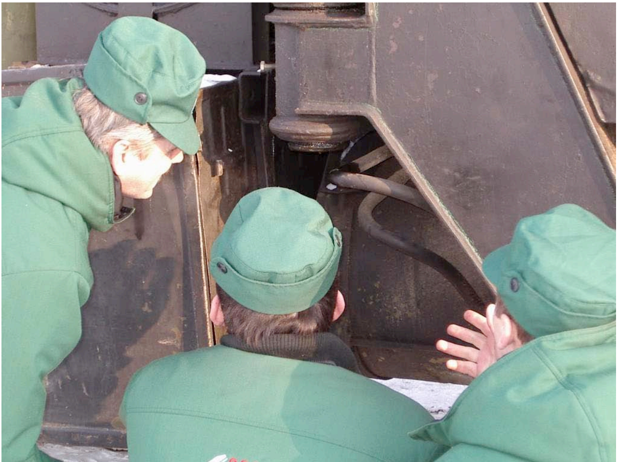
Figure 5.13: Crane Examination Techniques – Hydraulic Lines and Bearing Surfaces.
