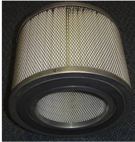
Figure 17. CBR/TIC HEPA Filter
