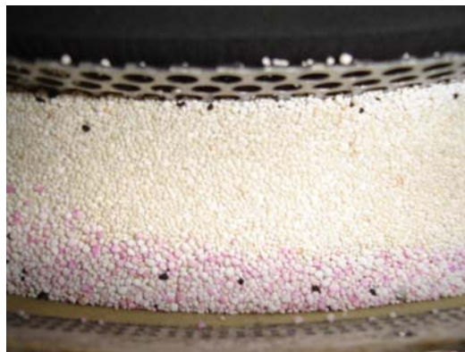
Figure 32. Pink Zeolite from Filter Disassembly
