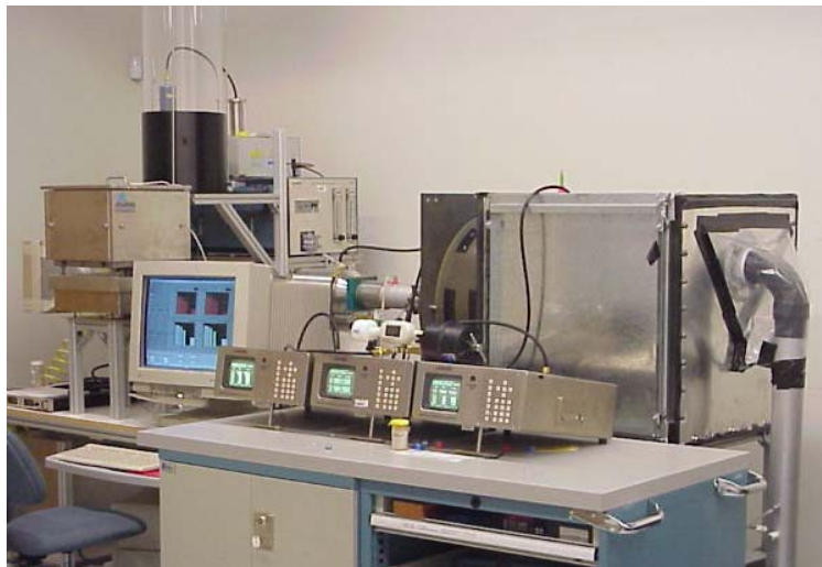
Figure 22. Filter Efficiency and Dust Capacity Test Stand
