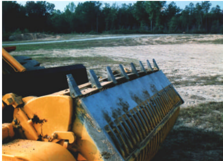
Figure 16. Blast Distortion (Bowing) to ROTAR ®
