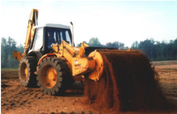
Figure 10. ROTAR ® Sifting Berm Soil
