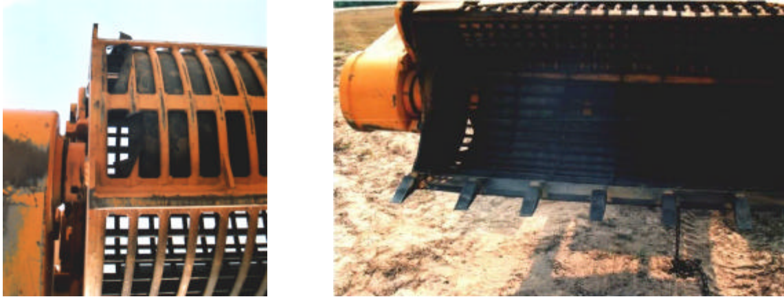
Figure 17. Blast Test Damage to Steel Liner
