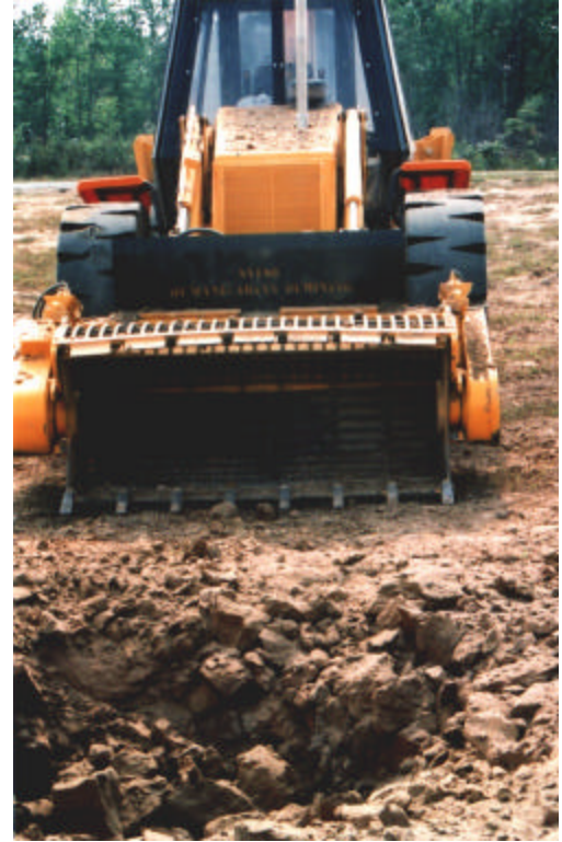
Figure 21. Improved Backhoe After AT Mine Detonation
