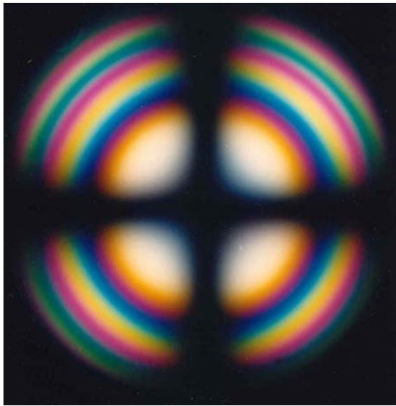
High-quality single-crystal sapphire dome viewed through crossed polarizers
