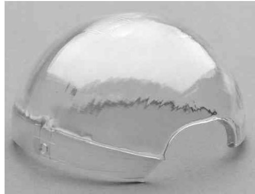
Figure 14: As-grown EFG sapphire produced by Saphikon. 19,20
