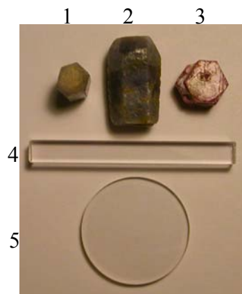
Figure 1: Natural sapphire (1, 2), natural ruby (3), and synthetic sapphire (4, 5).
