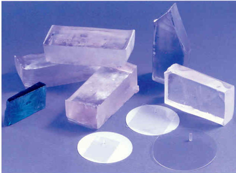
Horizontal directional solidification (Bridgman growth)
