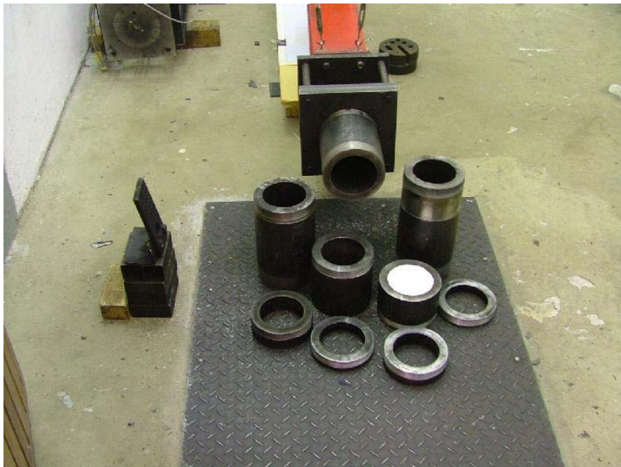
Figure 3: Different extension tubes can be attached to the test rig
