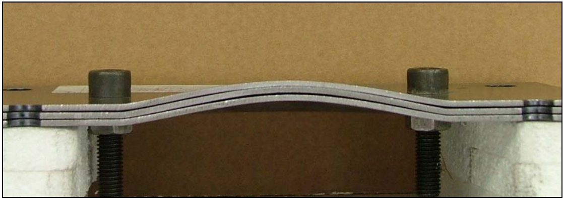
Figure 10: Photograph of plate profile for test plate subjected to same charge mass (5g) but different load conditions (LC-1, LC-2 and LC-3) Test plate Numbers, NJ210405a, NJ210405b, NJ210405c
