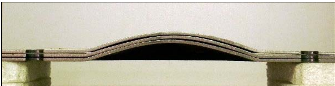
Figure 11: Photograph of plate profile for test plate subjected to same charge mass (7g) but different load conditions (LC-1, LC-2 and LC-3) Test plate Numbers, NJ220405c, NJ220405e, NJ220405f
