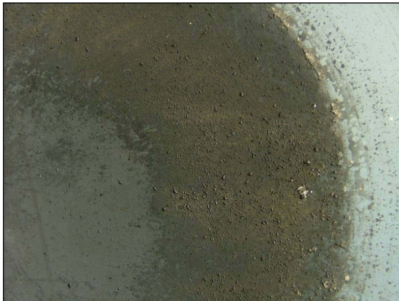
Figure 9: Photograph showing a close up view of the polystyrene residue visible for test plate (NJ210405c) subjected to load condition LC-3
