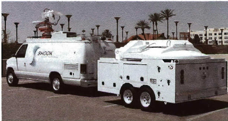
Figure 9. 2.4-meter transportable terminal. VertexRSI 240 DMVO antenna system mounted in a 240 AT trailer by Shook Mobile Technologies.
