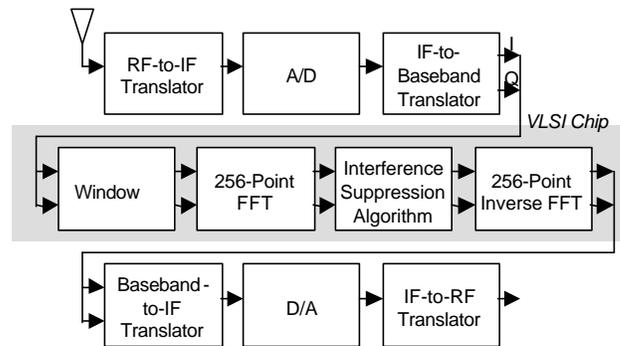
**Figure 1. Block Diagram of Applicqué Configuration**
