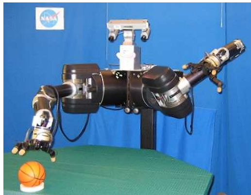
Fig. 1. Dexter, the UMass bi-manual humanoid.
