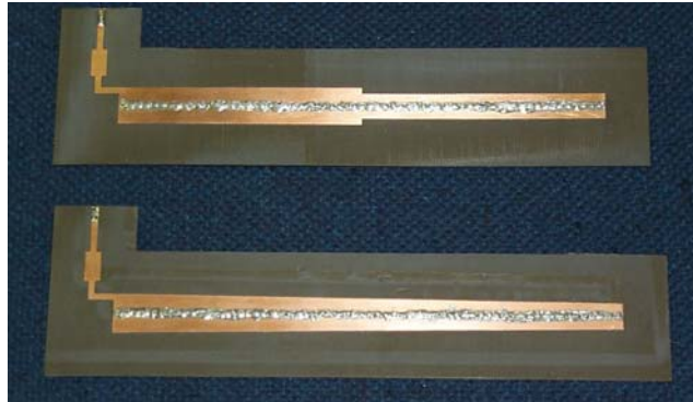
Figure 8: Stepped (top) and Sloped (bottom) arrangement of the “half-width” design fabricated and tested in RASCAL.
