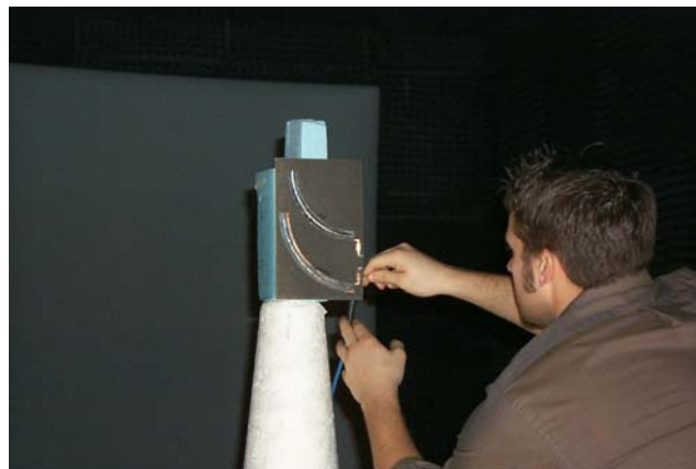
Figure 7: Curved arrangement of the “half-width” design fabricated and tested in RASCAL.
