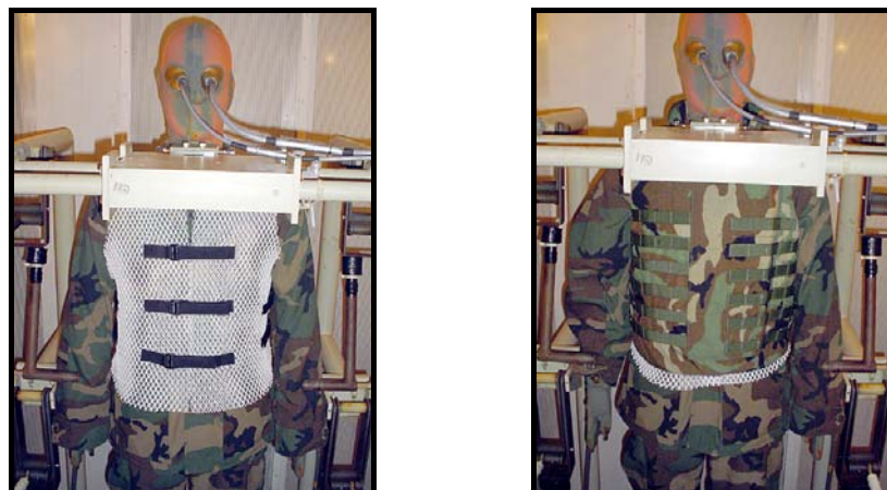
Figure 2. Photographs showing the thermal manikin (TM) configured with the Temperate Battle Dress Uniform (TBDU), and a spacer vest (SV, both left), and under the Interceptor Body Armor (IBA, right).
