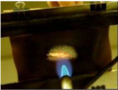
Figure 15. Foam After Five Minutes of Flame Exposure.
