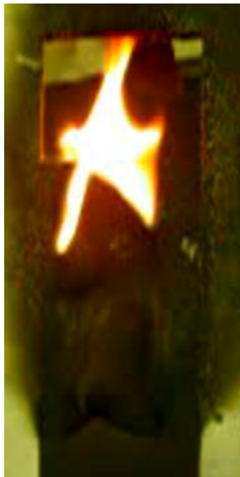
Figure 10. Examples of PVC/NBR Foam Failing Fire Screening Test (afterflame > 2 seconds).
