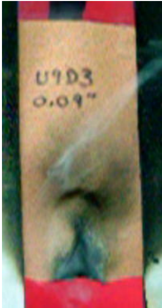
Figure 9. Examples of PVC/NBR Foam Passing Fire Screening Test (afterflame < 2 seconds).
