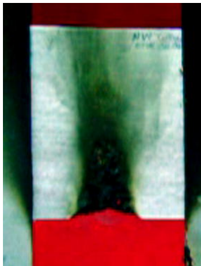
Figure 12. Screening Fire Test of Nonwoven and PVC/NBR Foam Composite.
