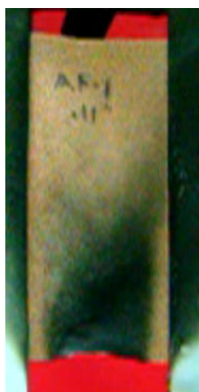
Figure 11. PVC/NBR Prototype Foam vs. Shelter Fabric After 12 Second Flame Exposure.
