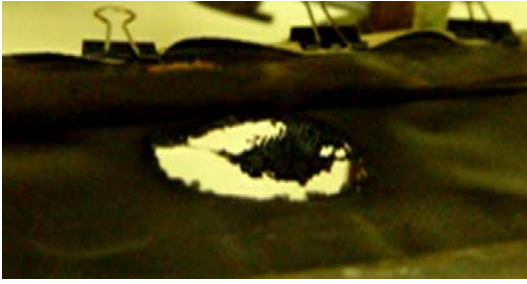
Figure 14. California Medium Shelter after 10 seconds of Flame Exposure.
