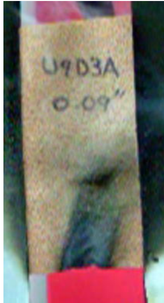
Figure 9. Examples of PVC/NBR Foam Passing Fire Screening Test (afterflame < 2 seconds).
