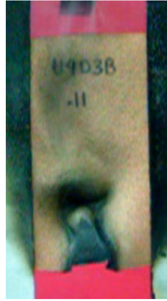
Figure 9. Examples of PVC/NBR Foam Passing Fire Screening Test (afterflame < 2 seconds).
