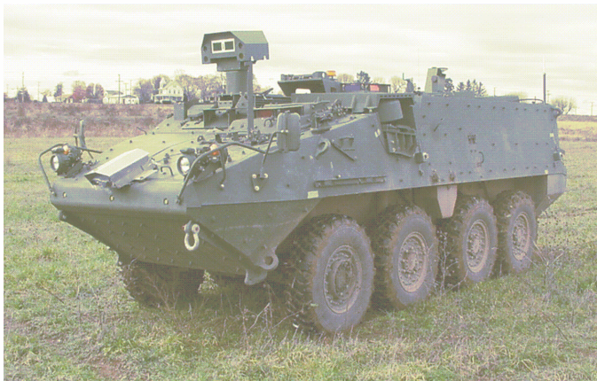
Figure 3. Robotic Follower based on Stryker Infantry Carrier Platform.
