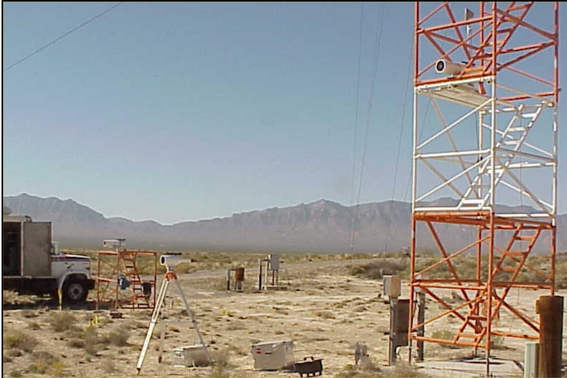
Figure 6. Two kilometer (2 km) scintillometers. ARL 2 m scintillometer is on scaffold at left. ARL 4 m scintillometer is at second level of scaffold at right. German scintillometer is on white tripod at left center.
