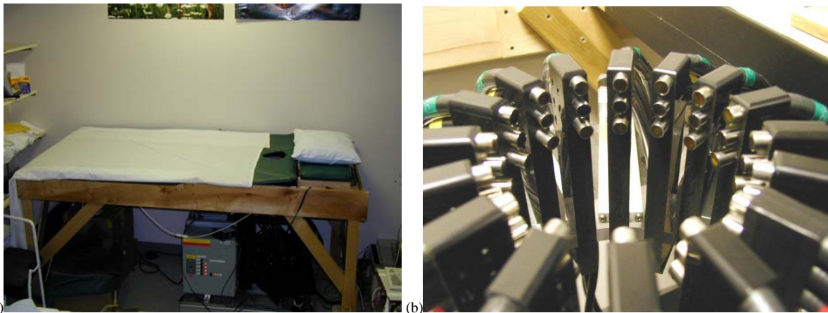
Figure 1. (a) The exam station with a single opening for the breast. (b) Optical fiber probe arrangement (16 equally spaced fibers at 3 separate levels, each level is separated by 10 mm) currently at use. The fibers can be opened or closed to suit each individual subject during setup. The breast is suspended through this opening, and optical fiber probes are brought into contact with the tissue surface.
