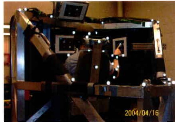
Figure 4: Motion Simulator Cab with Reflective Markers
