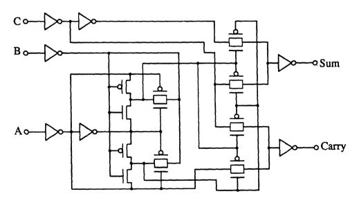
Figure 4-15: Three-bit adder circuit
