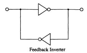
Figure 2-2: Cross-coupled inverter circuit.
