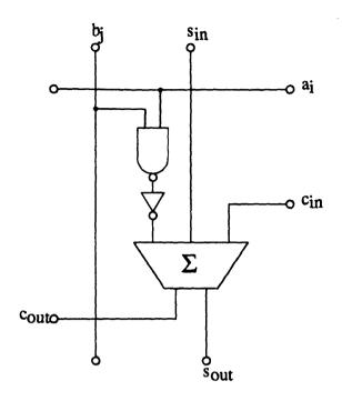
Figure 4-14: Array multiplier cell
