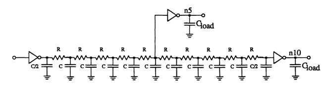
Figure 4-16: RC model for poly interconnect line
