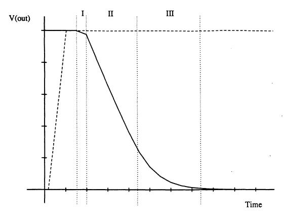
Figure 2-3: Output waveform of a CMOS inverter.
