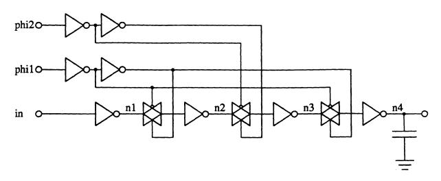
Figure 4-11: Shift register circuit.
