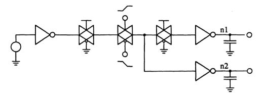
Figure 4-10: Circuit testing switching transmission gate model.
