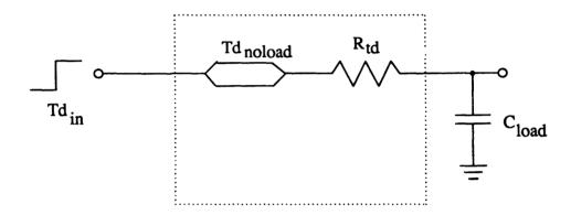
Figure 2-9: Model for delay calculation of a cell
