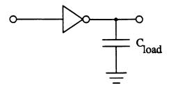
Figure 4-1: Inverter circuit.
