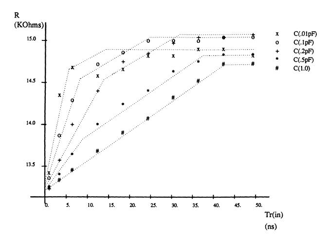
Figure 2-18: Conducting transmission gate effective resistance function.
