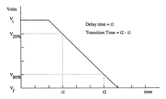
Figure 2-5: Ramp model of a waveform
