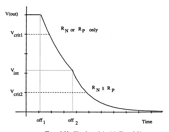
Figure 2-23: Waveform of circuit in Figure 2-21.
