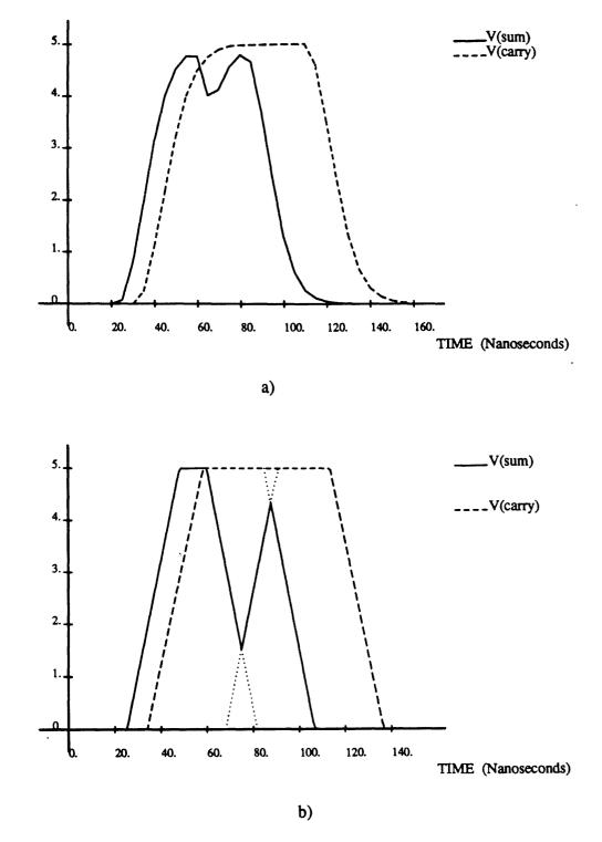
Figure 4-8: Output waveforms for the circuit of Figure 4-6.
