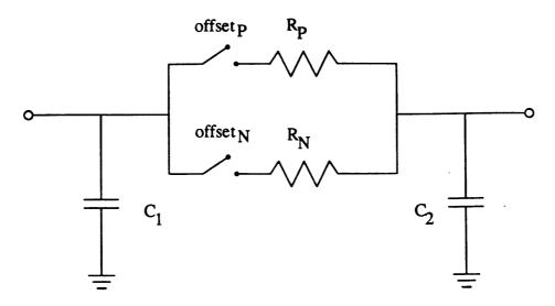
Figure 2-21: Switching transmission gate model.
