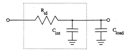
Figure 2-12: Model of a cell with internal delay modeled with a capacitor
