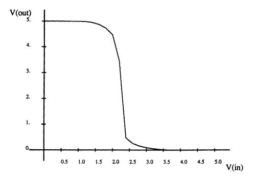
Figure 2-4: D.C. transfer function of a CMOS inverter.
