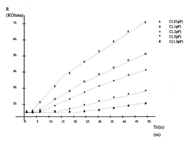
Figure 2-20: Switching transmission gate effective resistance function.
