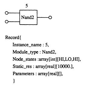
Figure 3-4: Instance representation of NAND gate module.
