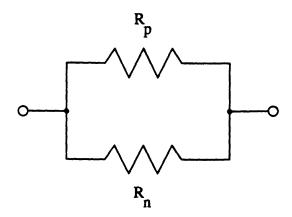
Figure 2-22: Resistance model of conducting transmission gate.
