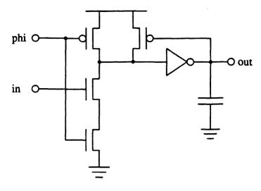
Figure 4-4: Domino logic test circuit.
