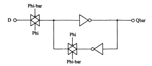
Figure 3-8: CMOS two phase flip-flop.
