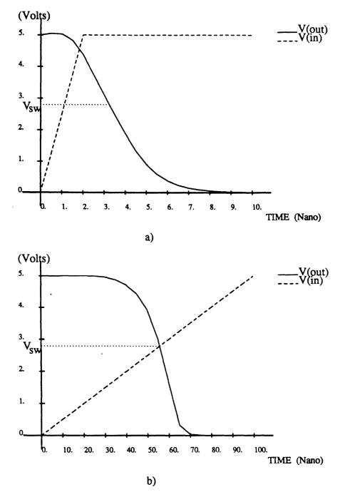
Figure 2-11: Effects of input transition on delay.
