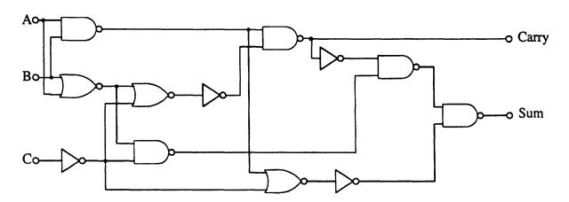
Figure 4-6: Logic gate implementation of a three-bit adder.
