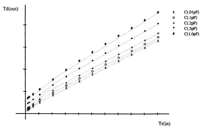
Figure 2-10: Output delay time function of an inverter.
