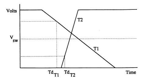
Figure 3-6: Closely spaced transitions with different transition times.
