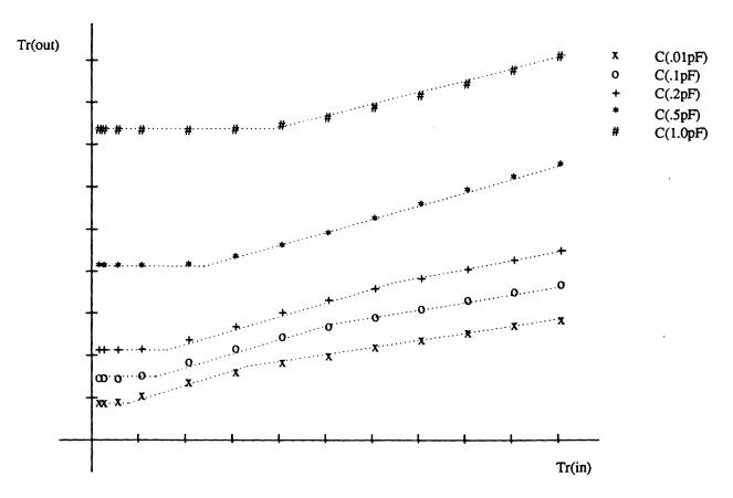
Figure 2-8: Output transition time function for an inverter.
