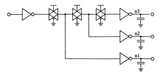
Figure 4-9: Circuit testing conducting transmission gate model.
