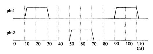
Figure 4-12: Clock waveforms for shift register.
