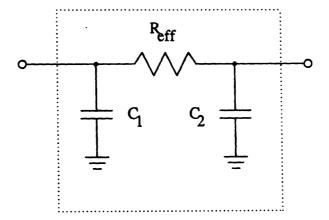
Figure 2-17: Model of conducting transmission gate
