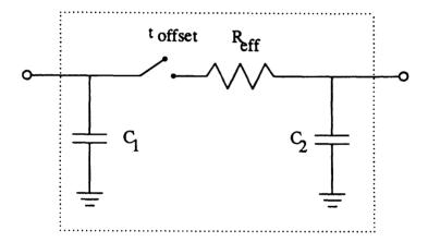
Figure 2-19: Model of switching transmission gate
