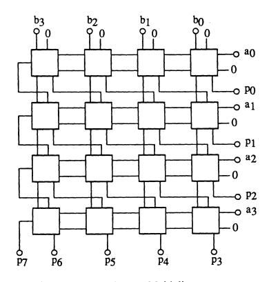
Figure 4-13: 4x4 Array Multiplier
