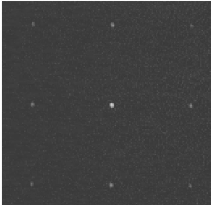
**Fig. 54.** Fan-out pattern from a single 970 nm VCSEL element within an  $8 \times 8$  array, transmitted through a 4:2:1 diffractive optical element (DOE).
