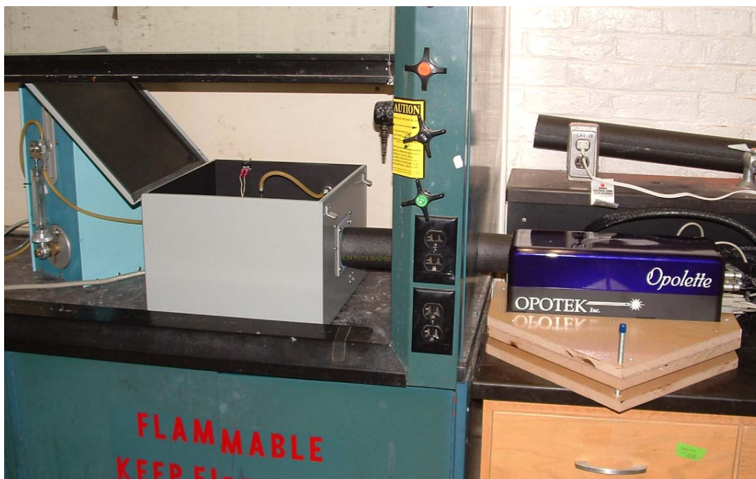
Figure 3. Automated batch reactor aligned with an Opotek, Inc. tunable UV laser source.
