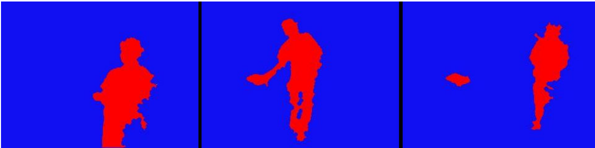
Figure 5.2: Background subtraction mask showing a human-object interaction. From the mask it cannot be decided whether the object has been deposited or removed. Although it may seem the opposite, in this case the object has been removed.
