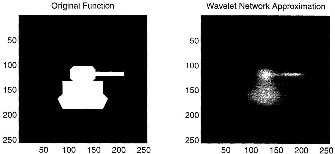
Figure 9: Wavelet network representation of simulated tank
