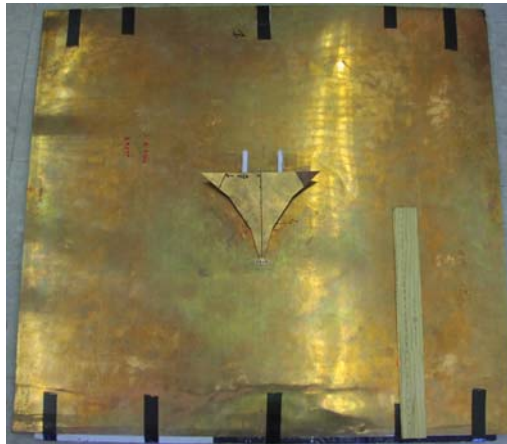
Figure 3: Fabricated tapered sector with bent corners.
