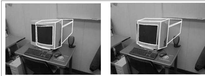
Figure 9. Pose refinement using the graduated assignment algorithm: initial pose (left) and final pose after applying the algorithm (right).
