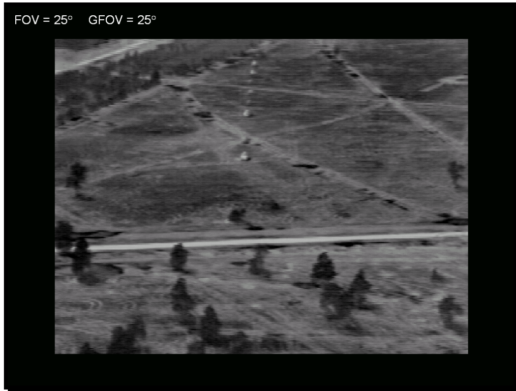
Figure 6. Representation of a forward-looking infrared sensor image from a 25° FOV sensor shown in a 25° FOV display.
