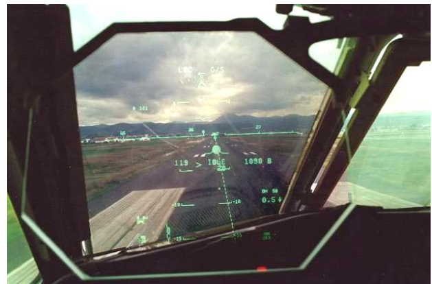
Figure 9. Image of the Head-Up Display symbology developed by Rockwell Collins.
