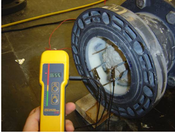
Figure 12. Taking moisture reading from test cell.
