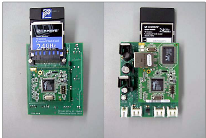
Fig. 5. Master (left) and slave (right) controller hardware. The master controls the wireless Ethernet.
