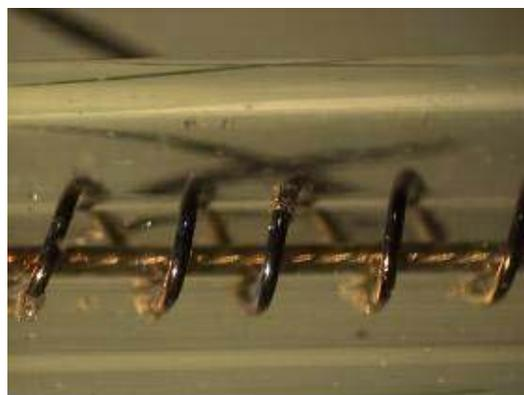
**Figure 4-5: 65  $\mu\text{m}$  PDMS HSA-SPME Device Before (Left) and After (Right) Sampling at a Flow Rate of 1.5 L/min.**
