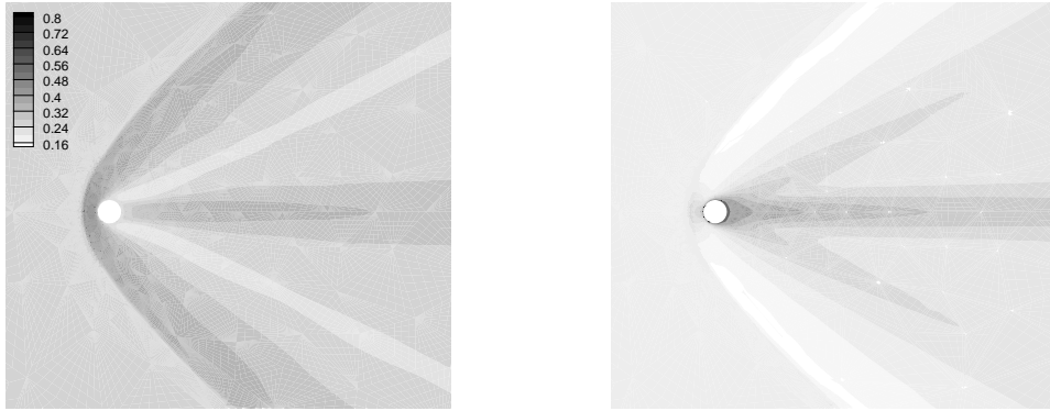
Figure 8: Instantaneous nondimensional temperature contours for flow past a circular cylinder at Mach number 2, Reynolds number 100 and cylinder wall temperature T_i = T_e = 0.225 . Left : Ion temperature contours. Right : Electron temperature contours.
